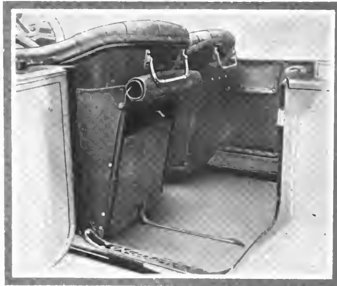
Method of concealing auxiliary seats on six-passenger body. They fold into the front seats and are covered by curtains
